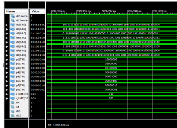
Fig. 9: SEC–DAEC (72, 64) per-bit joined-pattern correction optimization for the bits d10 and d12 Simulation Wave Forms.
