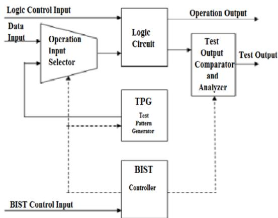
Fig. 1: Simple Block Diagram of BIST Design
