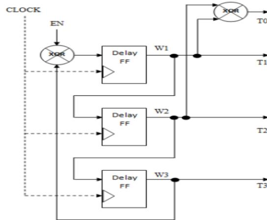
Fig. 3: Logic Diagram of Test Pattern Generator used in Proposed Design
