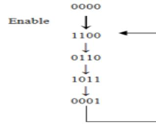
Fig. 2: Flow Diagram of Random Sequence Generation by TPG
