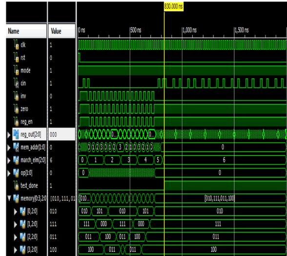
Figure 5: simulation results of BIST with March C algorithm with symmetric
