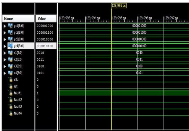
**Fig. 8: Output for the pipelining method**
