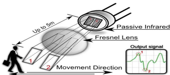
Fig:-2. Internal structure of PIR sensor
