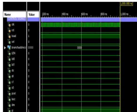
Figure 8.1: Control signals for Sequential FIR Filter
