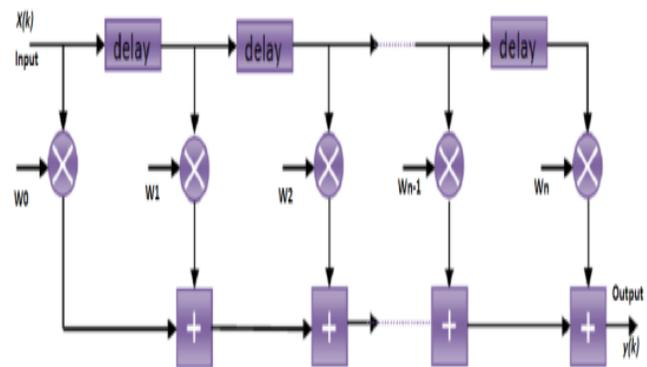
Fig 1: Direct form FIR filter
