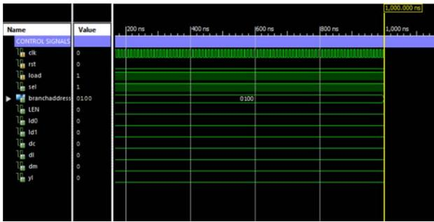
Fig 8.1 Control signals for Parallel FIR Filter
