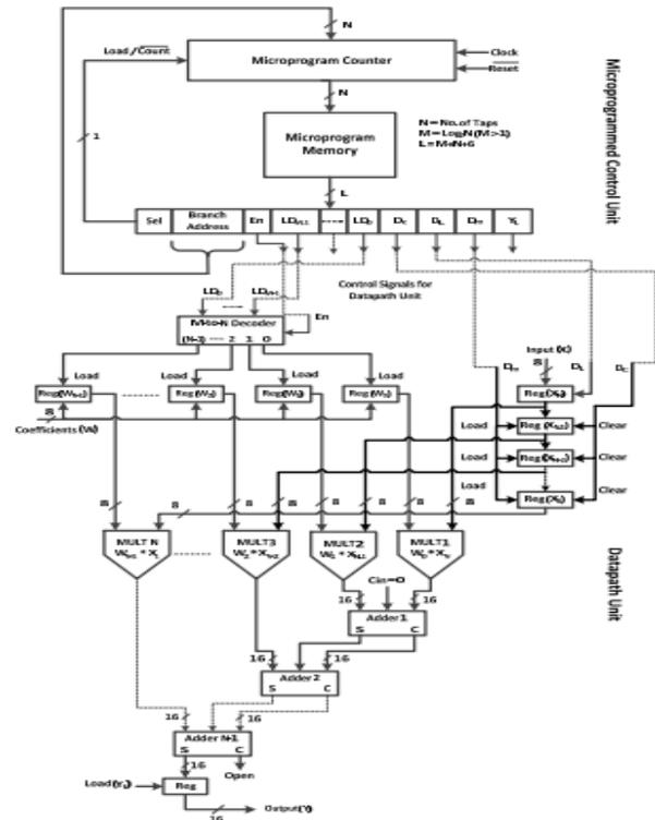
Fig 3: Architecture of parallel micro programmed FIR filter
