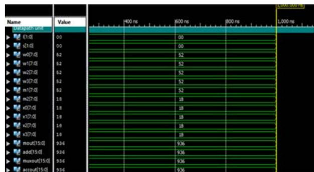
Fig.7.2 Data path unit of Sequential FIR Filter
