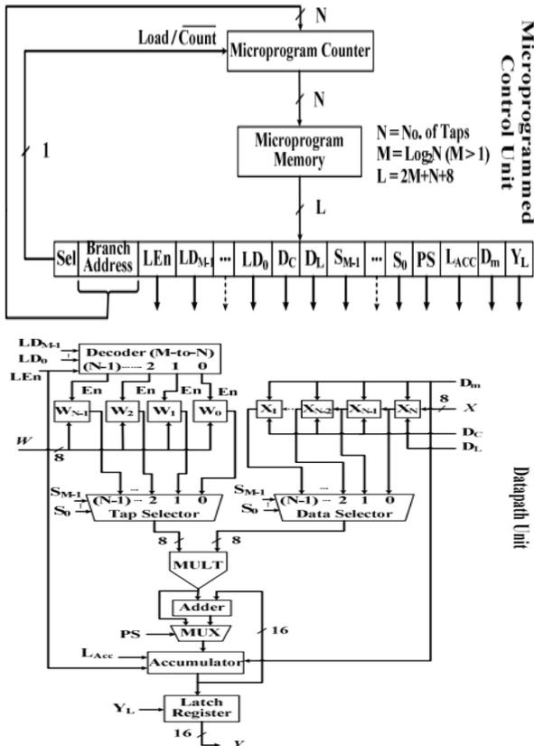
Fig 2: Architecture of sequential micro programmed FIR filter
