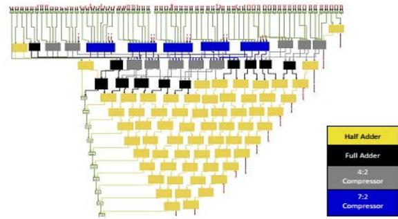
Fig. 6 Hardware architecture of Compressor based Urdhwa Multiplier
