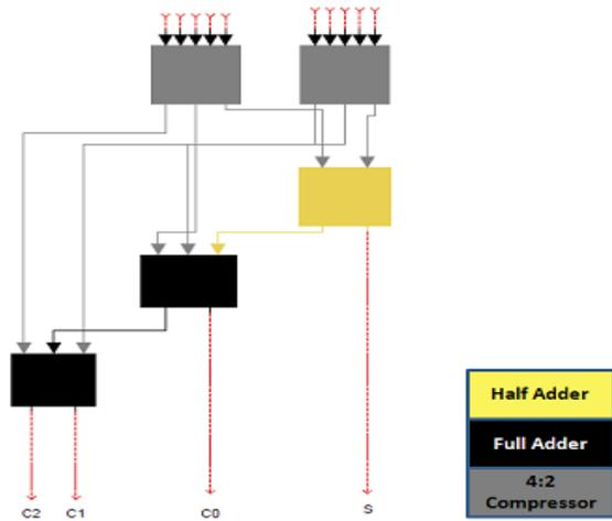
Fig 4: 4:2 Compressor using full adders and half adders
