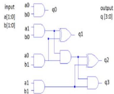
Fig. 4: Hardware realization of 2x2 Vedic multiplier
