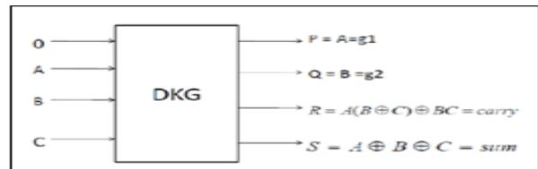
Fig.8 DKG Gate Working As The Full Adder
