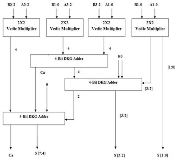
Fig. 5: Hardware realization of 4x4 Vedic multiplier
