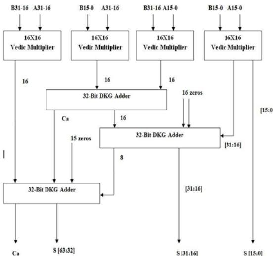
Fig.6: Hardware realization of 32x32 Vedic multiplier
