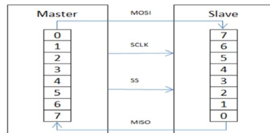
**Fig. 1 Data Transfer Type of SPI****A. Control Address**
