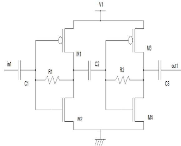
**Figure 2: Schematic of current reuse LNA**
