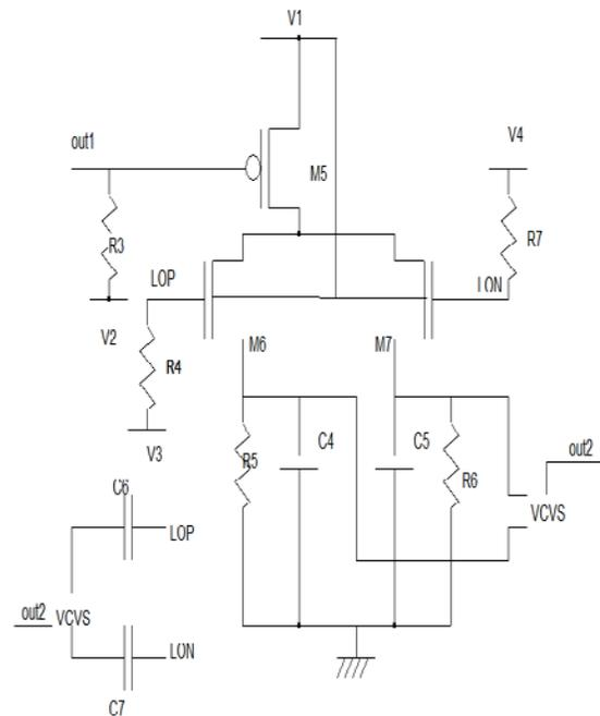
Figure 6: Schematic of Mixer
