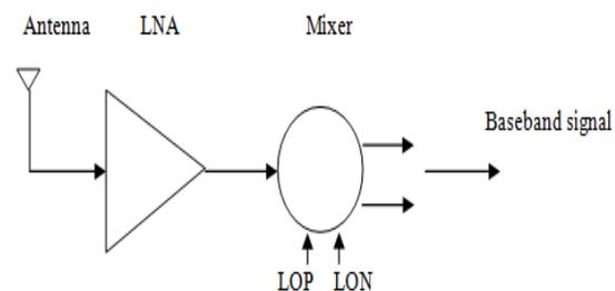
**Figure 1: Block Diagram of RF Front-end design of Digital TV Receiver**
