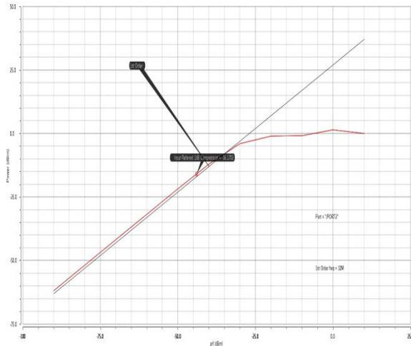
Fig.7 1dB compression point for Front-end of Digital TV Receiver
