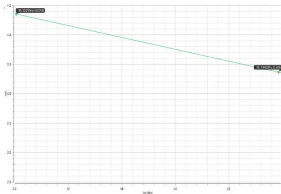
Fig.9 Conversion gain for Front-end of Digital TV Receiver
