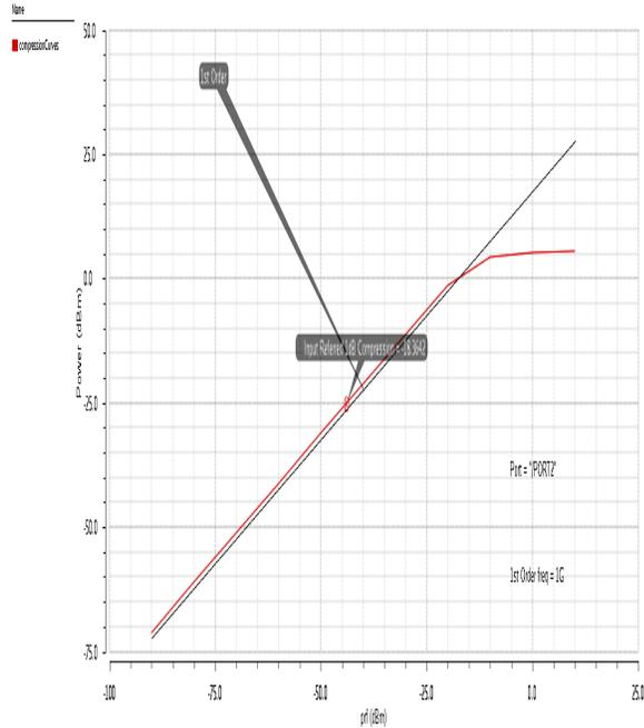
Figure 4: 1dB compression point of current reuse LNA
