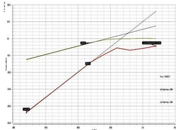
Fig.8 Input-referred third-order intercept point (IIP3) for Front-end of Digital TV Receiver
