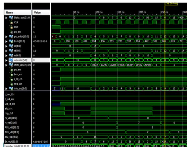
Figure 6.1: 6 Stage pipeline RISC results
