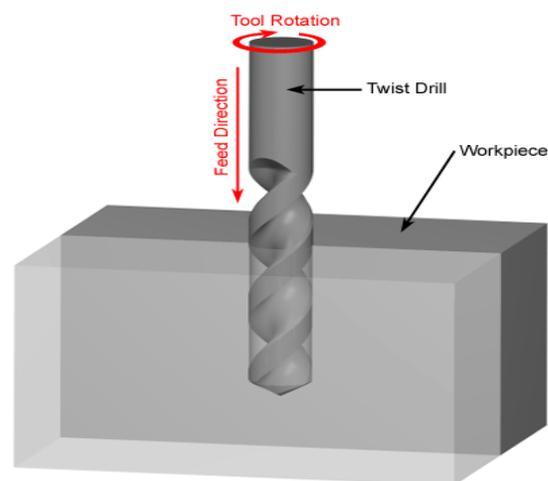
Figure 1: Drilling process
