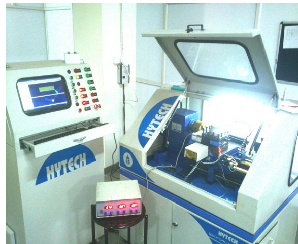
Figure 1: CNC lathe used for the turning purpose
