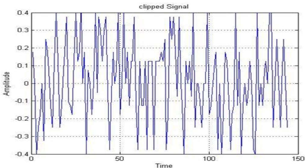
Figure: 3 Signal with clipped peak value
